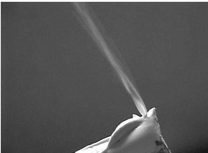
Laboratory simulation of chunna packet bursting on contact
