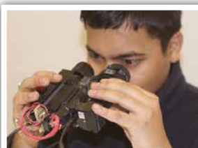
Owl: An ultra low-cost retinal imaging tool which uses machine learning algorithms to detect and quantify the presence of diabetic retinopathy.
